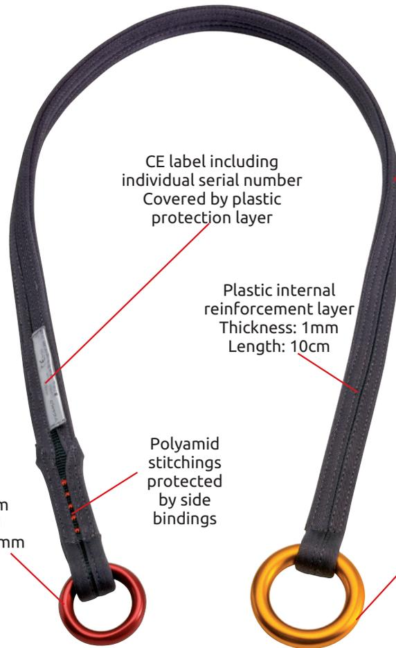
Double-layer polyester webbing with double side bindings for best stiffness and wear-and-tear resistance
