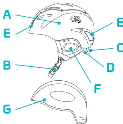
EN: (A) PC and PS composite shell, (B) PA chin strap with buckle, (C) PA size adjustment system, (D) PA harness, (E) PA lamp stop, (F) Earmuff optional, (G) Under-helmet optional.
