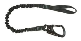
Designed for special ops personnel, this tactical tether connects the wearer to an anchor point in an aircraft or an edge. Made from 1-in tubular web with a built-in bungee, the Tactical Tether retreats as needed to stay out of the way. Girth hitch to attach the loop end to your harness and connect the other end to the anchor of your choice. Sewn to a black double-locking connector. Rated strength: 11 kN (2,473 lbf)
