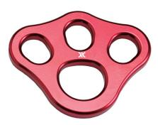
When weight and size are an issue, such as in mountain rescue and special operations packs, river rescue gear bags, or rope access work, the ultra-compact, light, anodized aluminum Micro-Anchor Plate is the right choice. The large hole acts as a collection point for multi-point anchors. The small holes keep carabiners separated, making them easier to work with when the system is loaded, and the oblong shape makes inserting carabiners easier and quicker.
